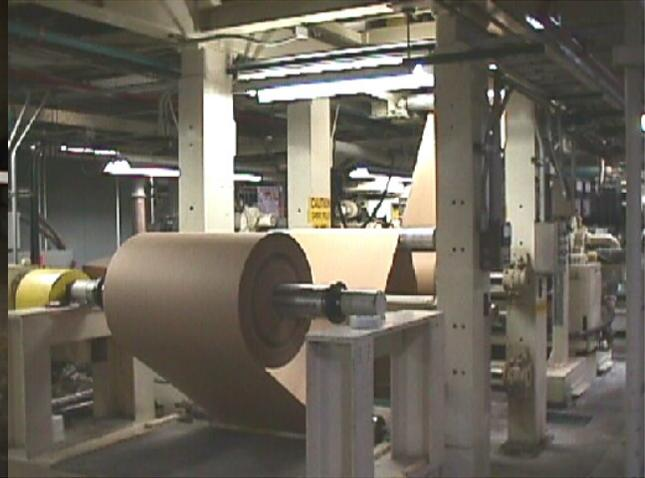
**Figure 21 - View of unwind station of the pilot coater**
