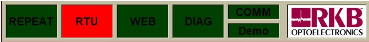
Figure 60 – System Diagnostics Alarm Indicators (show reel turn up alarm indication)
